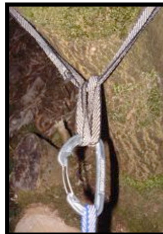
▲ Here we see a snap gate carabiner with gate interference causing the gate to open. Here is where a screw gate carabiner should have been used
