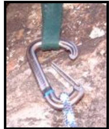
▲ Here we see a snap gate carabiner with gate interference causing the gate to open. Here is where a screw gate carabiner should have been used
