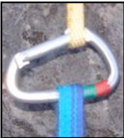
▲ Here we see cross-loading of a snap gate carabiner
